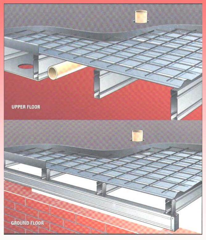
SYSTEM COMPRISES 70MM THICK SLAB FORMED ON COATED STEEL DECKING SUPPORTED BY ZINC COATED STEEL JOISTS
